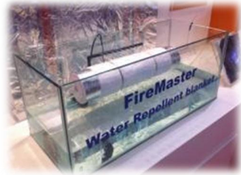
Firemaster Marine Plus used for Pipe lag and underside of Helicopter Platform
