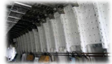
Firemaster Marine Plus used for bulk head; faster installation and overall customer preference
